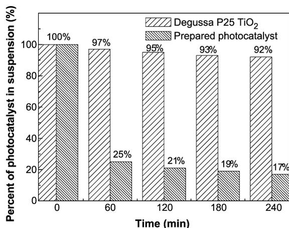
Fig. 8. The comparison of the precipitation percentage between Degussa P25 TiO<sub>2</sub> and prepared photocatalyst.
