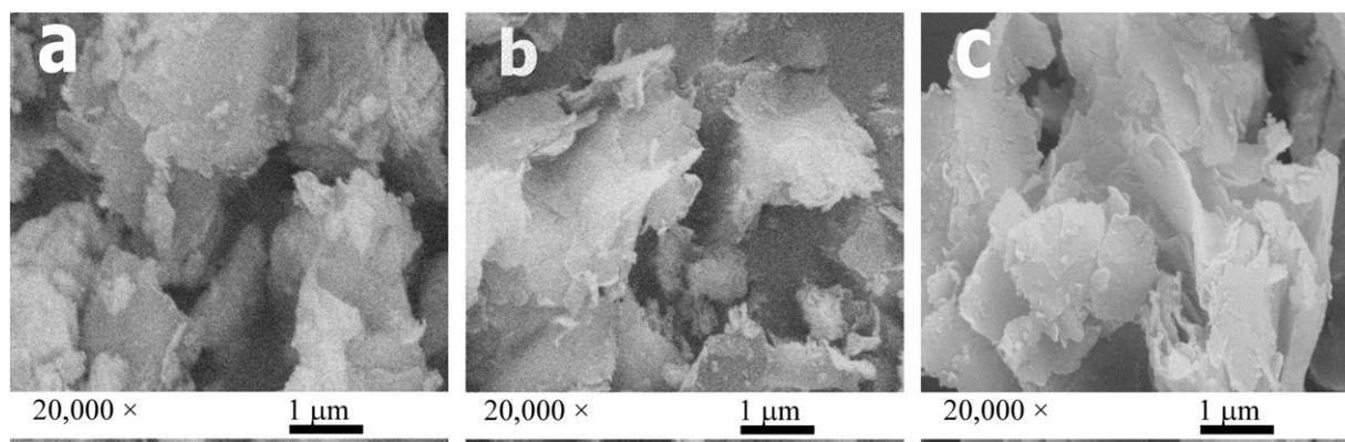
Fig. 2. SEM micrographs of Pt-MCHA pillared clays (a: 0.1%; b: 0.2%; c: 1.0% Pt).
