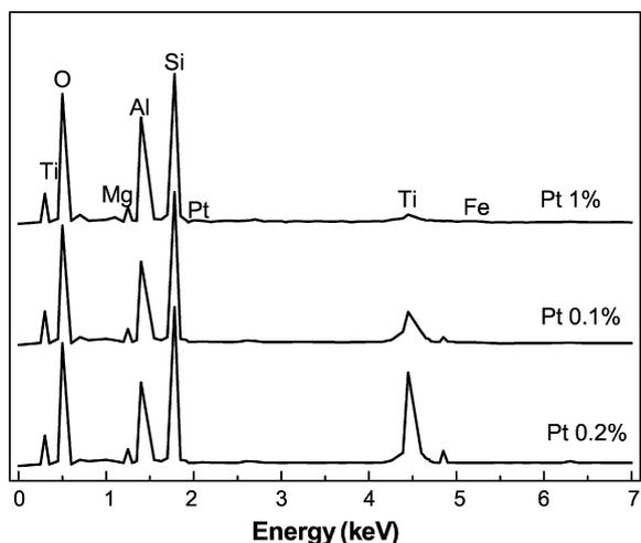
Fig. 5. EDX spectra of different pillared clays.
