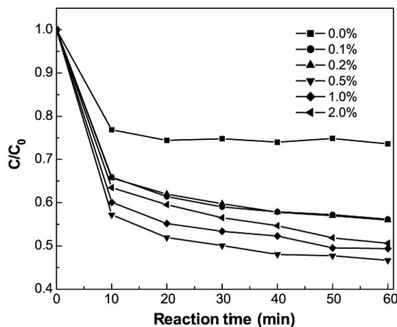
Fig. 9. Adsorption kinetics of MO using different Pt-MCHA pillared clays as adsorbents (the Pt concentration is indicated in the figure).
