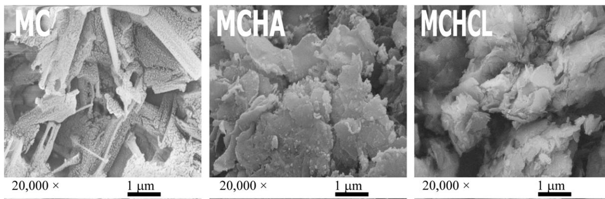
Fig. 1. SEM micrographs of raw MC, MCHA, and MCHCL clays.
