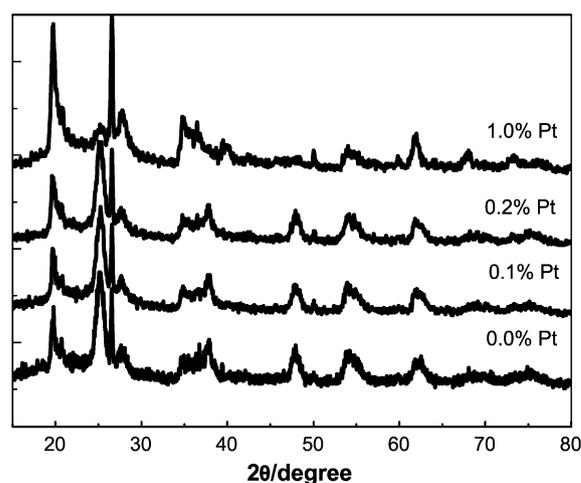
Fig. 4. XRD patterns of different Pt-MCHA clays.
