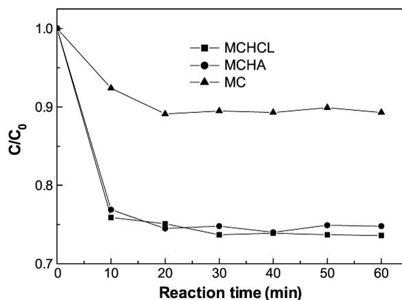
Fig. 6. Adsorption kinetics of MO on MC, MCHA, and MCHCL pillared clays.
