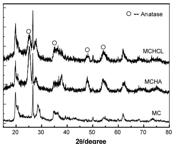
Fig. 3. XRD patterns of raw MC, MCHA, and MCHCL clays.
