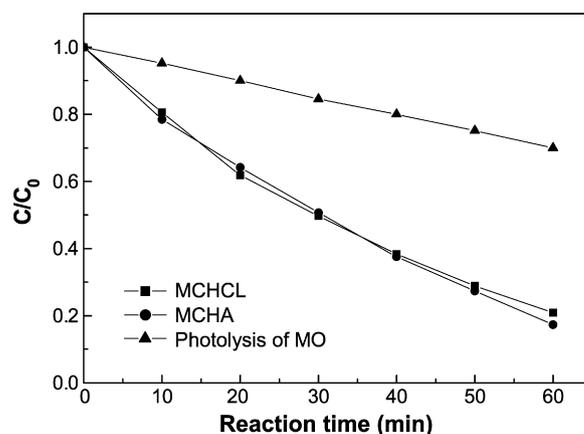
Fig. 7. Photolysis of MO and photocatalytic degradation of MO on MCHA and MCHCL pillared clays.
