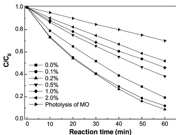
Fig. 10. Degradation kinetics of MO using different Pt-MCHA pillared clays as catalysts (the Pt concentration is indicated in the figure).
